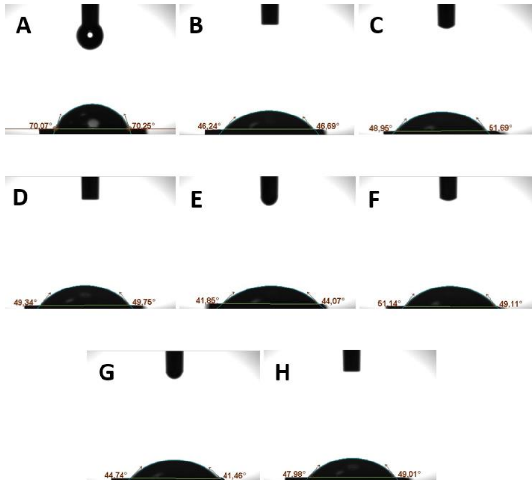
Figure 8.1: Water contact angles of plasma treated PLLA composite materials. A) 0 s, B) 30 s, C) 45 s, D) 60 s, E) 90 s, F) 120 s, G) 150 s, H) 180 s CAP treated PLLA composite materials.
